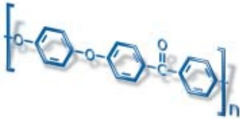
The base polymer has a melt viscosity of 100–3,000 Pas, measured at 400 °C, and a low shear of 1 sec<sup>-1</sup>, which is right for injection-molding and extrusion applications.
